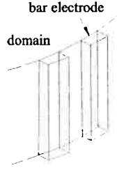
Fig. 2. Bar electrode attached to the conductive domain.
