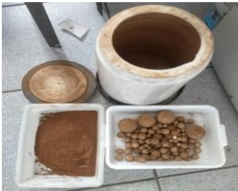
Figura 13: As fibras após as 72 horas no moinho de bolas
