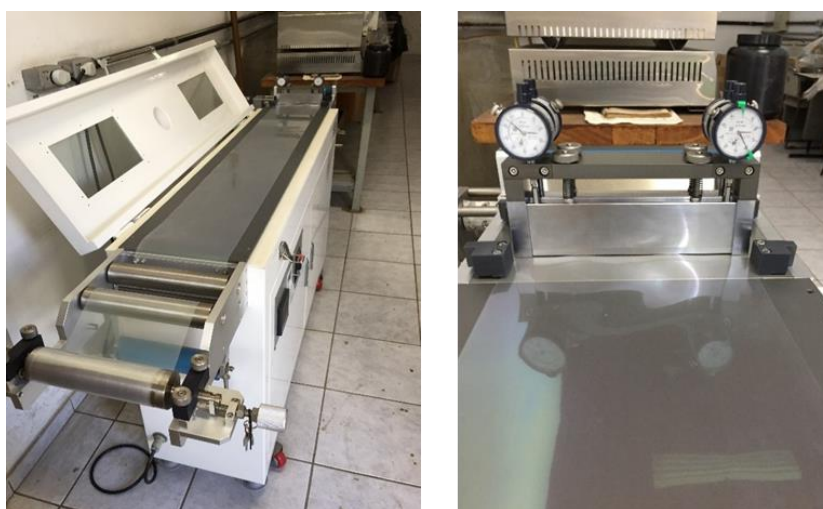
Fig. A1.1 Tape casting system (left) and doctor blade (right).
