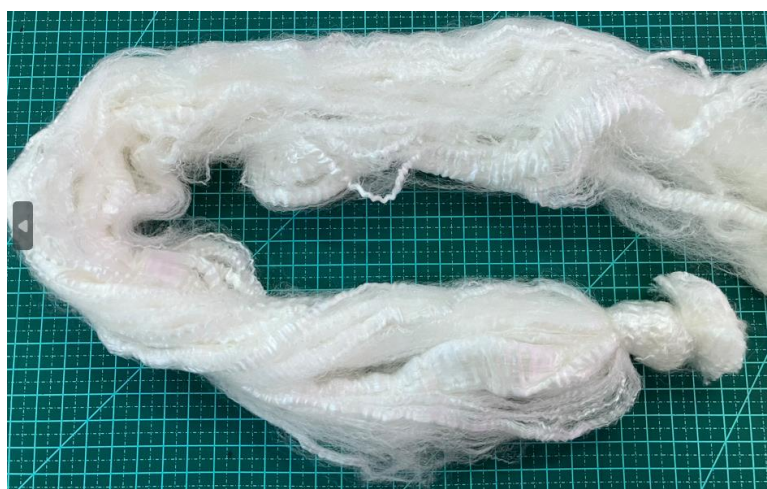
Figure 12 - Textile PAN-based fiber (5.0 dtex) supplied by JMHP Carbon
