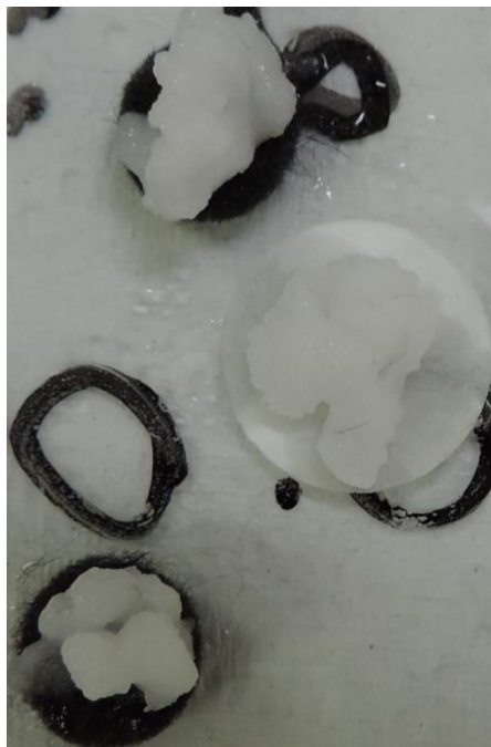
Figure 24 - Activated carbon fiber-felt (ACFF) electrodes and a qualitative filter paper (separator) impregnated with potassium hydroxide-glycerol hybrid electrolyte (KOH:GLY) before the diffusion process at room temperature
