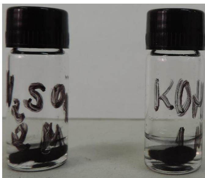
Figure 23 - Activated carbon fiber-felt (ACFE) electrodes immersed in acidic and alkaline aqueous electrolytes
