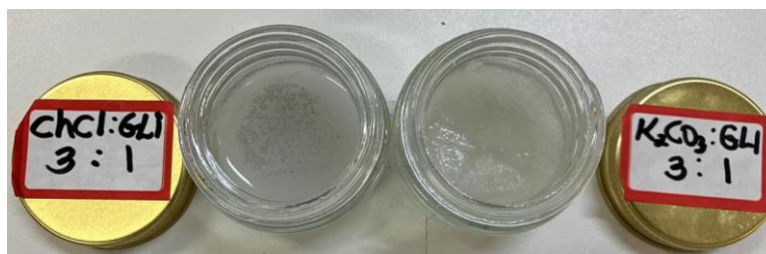
Figure 22 - ChCl:GLY (Choline chloride-glycerol hybrid electrolyte) and K_2CO_3 :GLY (Potassium carbonate-glycerol hybrid electrolyte) at a molar ratio of 3:1
