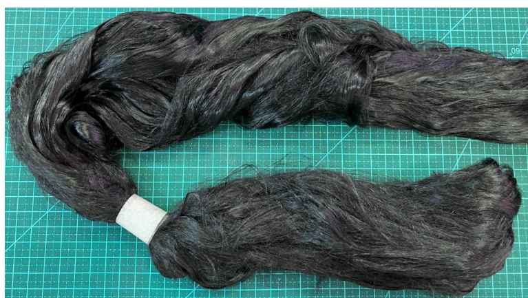
Figure 13 - Oxidized textile PAN-fiber
