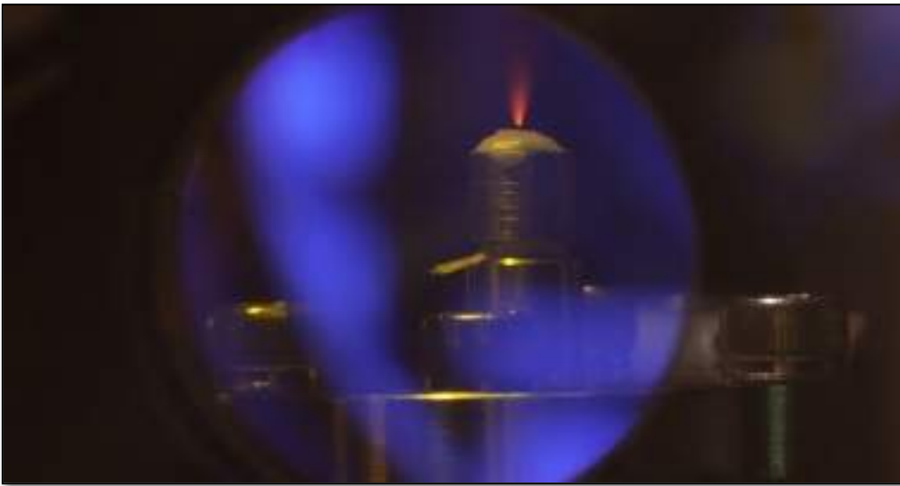
Figure 6.22 – Helium gas jet produced by a de Laval nozzle in vacuum, exhibiting a plasma excited by an ultrashort pulse. The jet shape can be observed by the light emitted by helium moving at supersonic speeds out of the laser interaction region.
