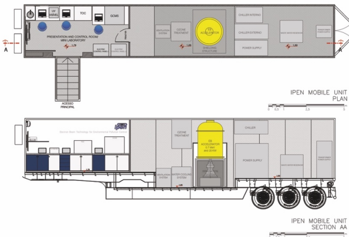
Figure 1 – Architectural design of the mobile electron beam irradiation unit.
