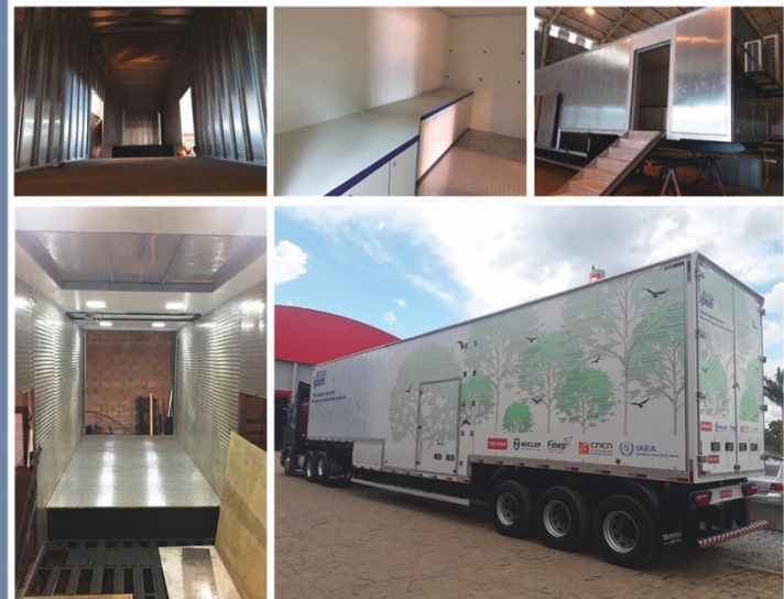
Figure 3 – Construction of the mobile electron beam irradiation unit.
