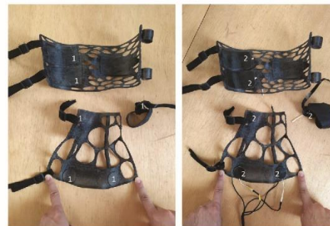
Fig. 4 3-piece shell of the wearable. 3D printed shell interior with embossed locations in the shape of the electrodes (1) for their precise positioning to the drinking FES training and (2) self-adhesive electrodes positioned.
