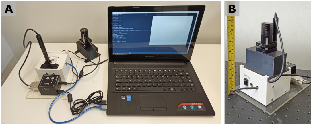
Figure 18 – Multiheight lens-free holographic microscope (a) connect to a laptop computer and (b) the equipment itself.
