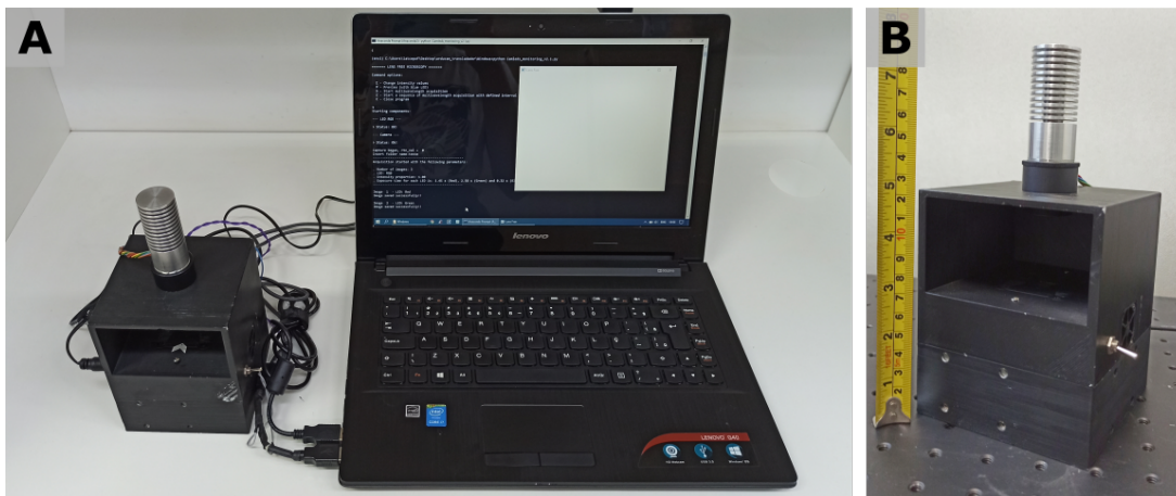
Figure 21 – Multispectral lens-free holographic microscope (a) connect to a laptop computer and (b) the equipment itself.
