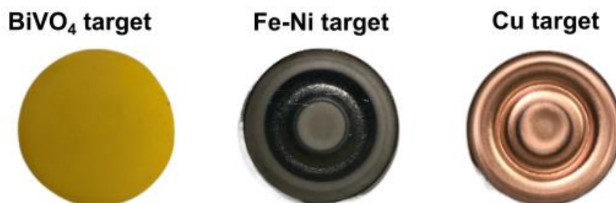
Figure 14 – Digital photographs of the (as-prepared) BiVO 4 , Fe-Ni, and Cu-target. The circular paths formed on the surface of the targets after magnetron sputtering deposition are the tracks left behind by secondary electrons under the influence of orthogonal magnetic and electric fields.
