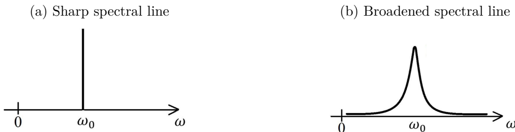
Figure 2 – Representative illustration of optical two-level transitions. In figure (a), it is represented the absorption or emission spectrum without line-broadening mechanisms so that we can assume the line shape g(\omega) = \delta(\omega - \omega_0) . In figure (b), it is represented the absorption or emission spectrum taking line-broadening mechanisms into account.
