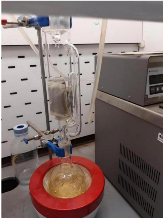
Figure 4-1 - Extraction from lignocellulosic biomass using Soxhlet equipment Source: By the author
