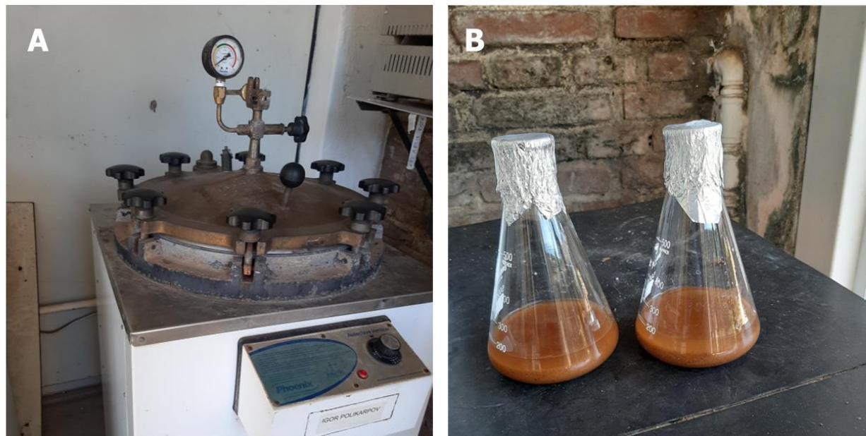
Figure 4-3 - Autoclave utilized for Lignocellulosic Biomass Pretreatment (A), LHW Autoclaved SCB (B) Source: By the author
