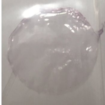
Figure 15 - Hydrogel of cellulose casted with chitosan reacted with ninhydrin. The purple color at the edges indicates the interaction between chitosan and cellulose.
