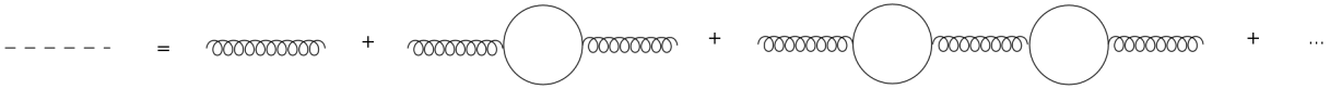
Figure 8 – Corrections to the gluon propagator due to light-quark loops, yielding the leading- n_f terms. Each bubble loop counts as n_f\alpha_s .
