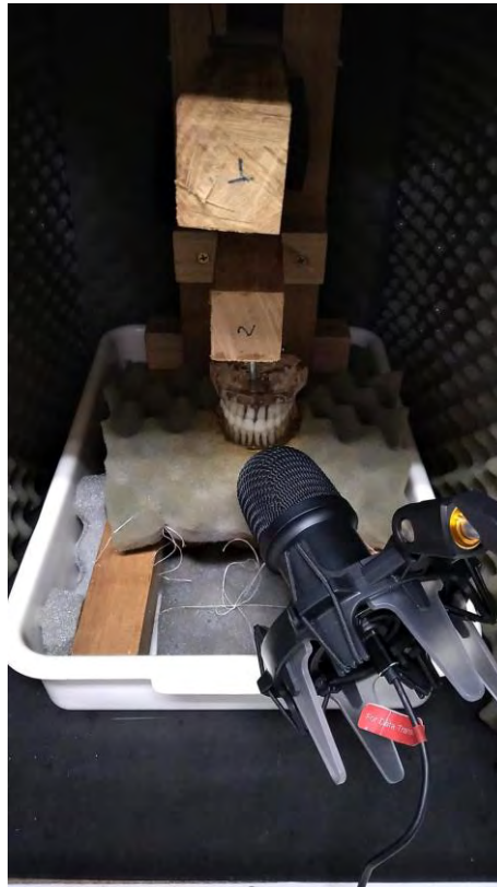
Figure 3.2: Crock Tester made of a wooden swing arm, a dental prosthesis, and a noise suppression box.
