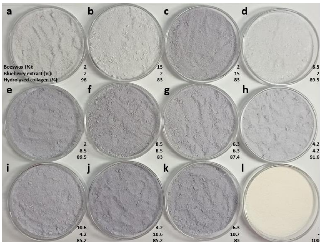
Figure 1 – Physical appearance of microparticles formulated with different percentages of beeswax, blueberry extract and hydrolysed collagen (% , % , %): (a-j) experimental runs, (k) optimised coated microparticles, and (l) pure hydrolysed collagen
