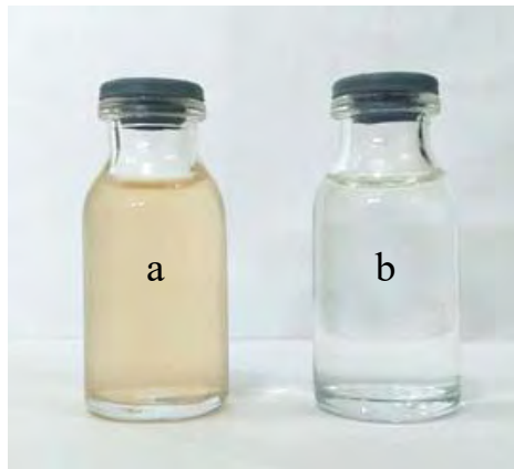
Figure 36 - Post-hydrothermal liquefaction wastewater values prior to (a) and after (b) the photocatalytic treatment
