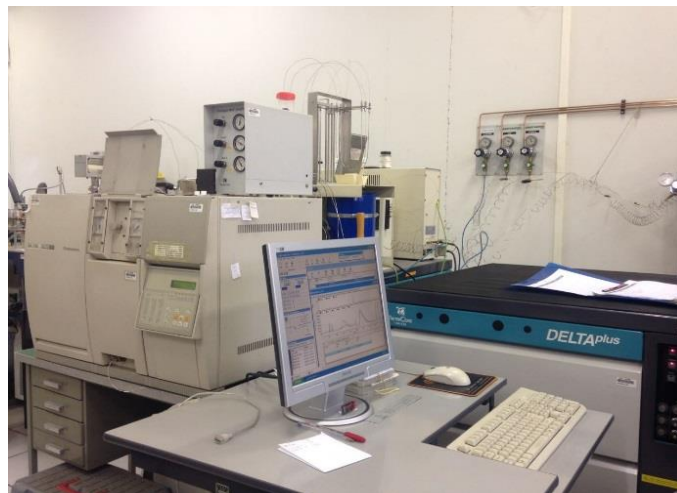
Figure 15 - Stable Isotopes Analysis performed in Continuous Flow Isotope Ratio Mass Spectrometry (CF-IRMS)
