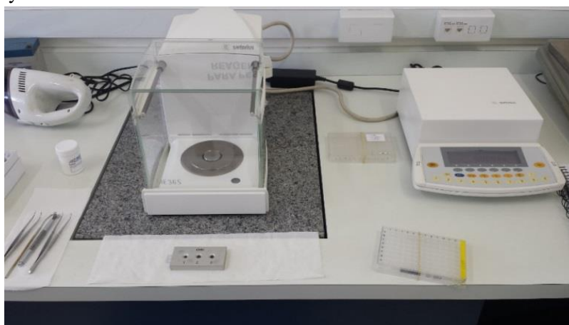
Figure 13 - Preparation for Stable Isotopes Analysis with dried material weighed in a precision analytical balance
