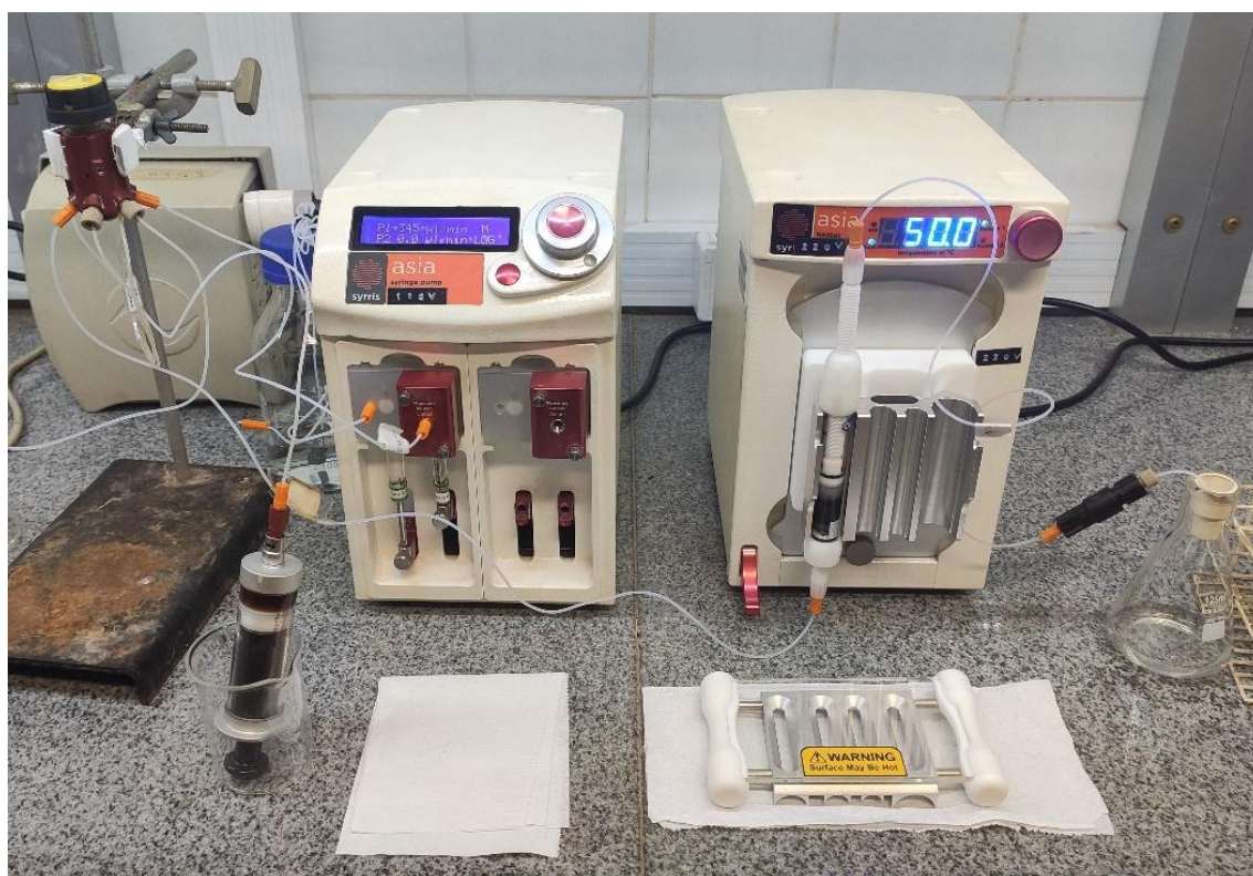
Figure 7. Our own Flow Asia system (Syrris) comprised of syringe pumps (left) and column heater with an exposed Pd/C-filled packed bed reactor (right).
