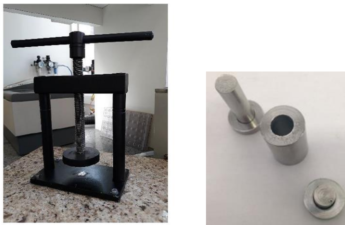
Figure 12. Manual press (on the left) and cylinder holder (on the right) used for salt-supported DBS preparation
