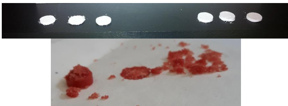
Figure 18. Comparison between tablets made of sodium sulfate (left), sodium carbonate (right) and sodium chloride (down) showing the mechanical instability of sodium sulfate and NaCl tablets.
