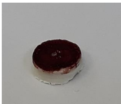
Figure 20. An example of an alternative salt-supported DBS containing blood spotted onto the sodium carbonate tablet.
