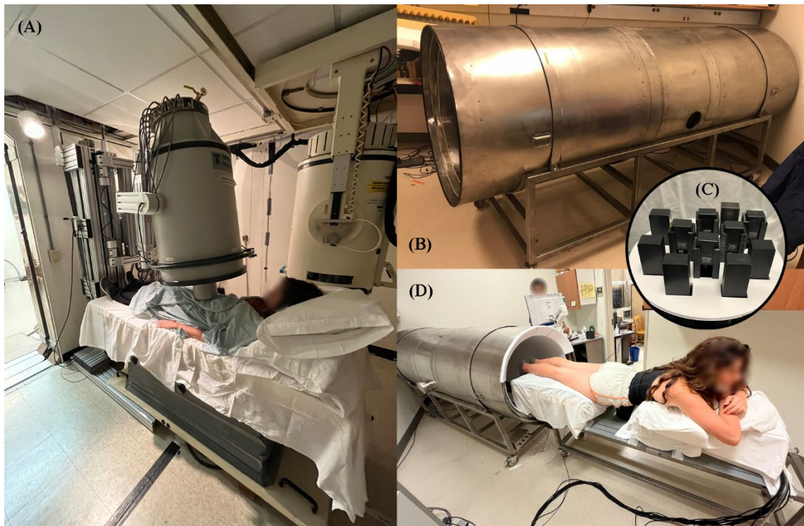
Figure 10 Pictures taken from the system installed at the University of Wisconsin-Madison. (A) SQUID in a cubic MSR. (B) Person-sized cylindrical shield. (C) Patient positioning for OPM-fMCG in the person-sized shield.
