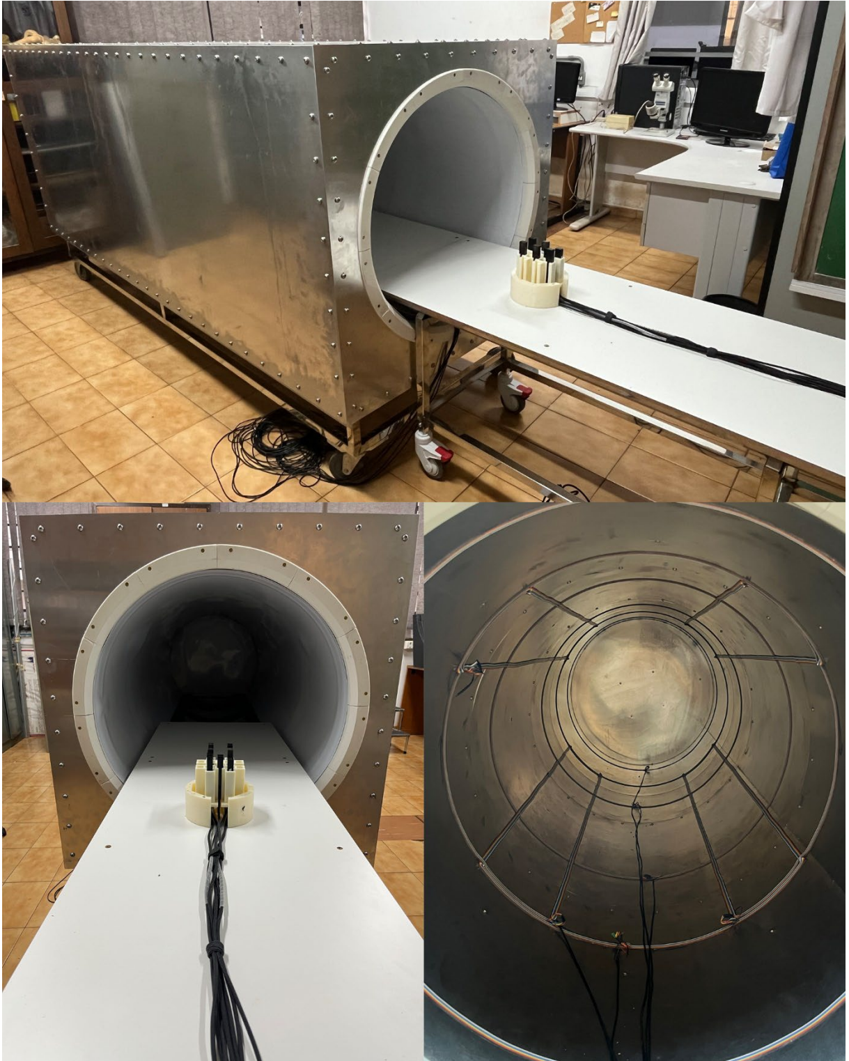
Figure 18 Person-sized magnetic shield installed in the Biomagnetism Laboratory at the University of São Paulo in Ribeirão Preto.
