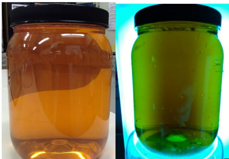
Figure 1.2: 15cm cylinder diameter and 12cm tall filled with FXO gel dosimeter; Left: non-irradiated; Right: Irradiated at the central portion with 3 Gy PDD max dose.
