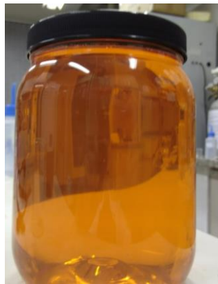
Figure 4.1: Cylindrical object (12.5 cm tall and 15 cm in diameter) filled with FXO-f to perform 3D dosimetry.
