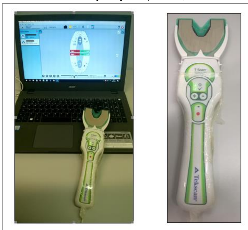
Figura 6 - T-Scan® III Occlusal Analysis System (Tekscan, Inc. South Boston, MA. USA)
