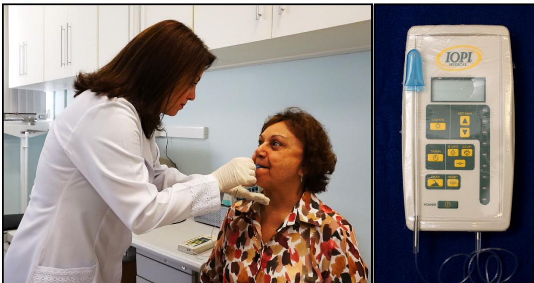
Figura 5 - Iowa Oral Pressure Instrument (IOPI) modelo 2.3.
