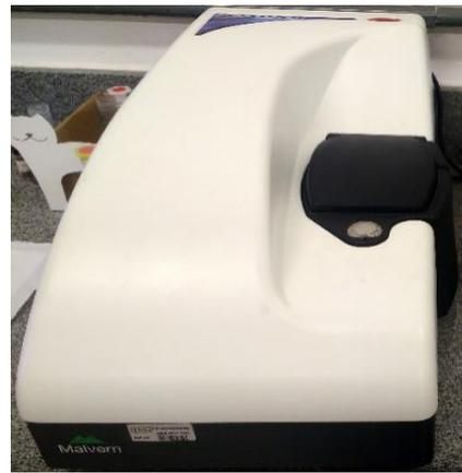
**Figura 2** - ZetaSizer Nano (Malvern Instruments Ltd)
