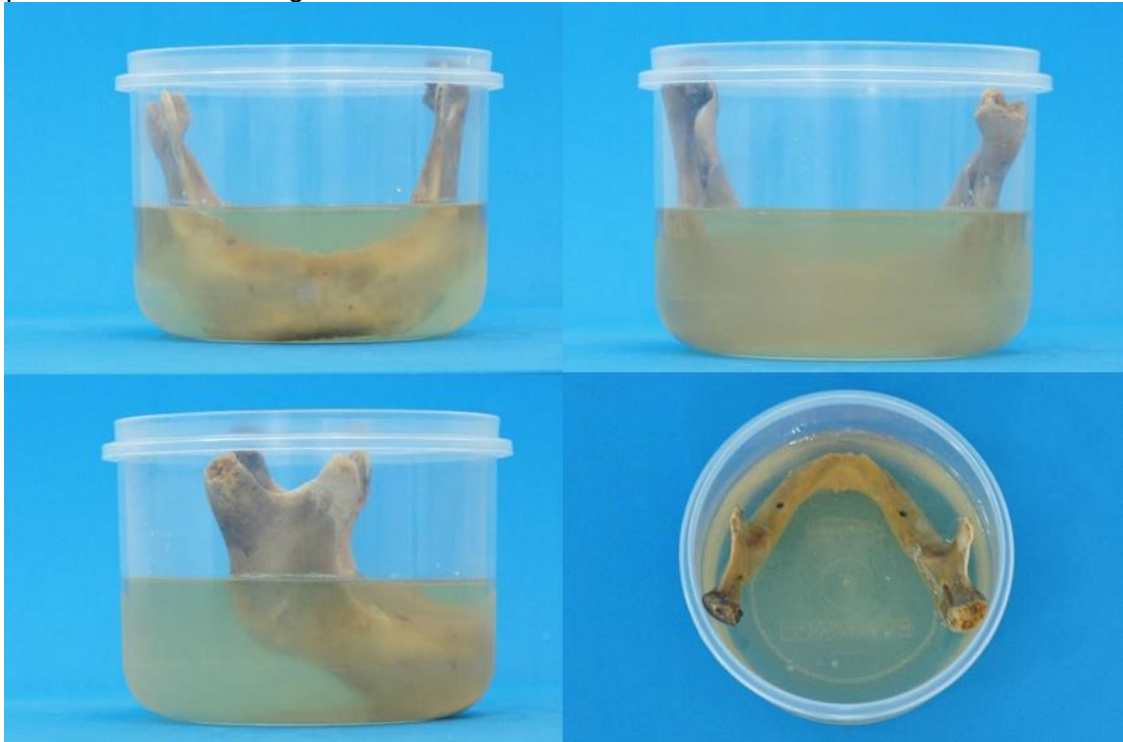
Figure 4. Phantom made from the mandible positioned in the center of a cylindrical plastic box in ballistic gelatin.
