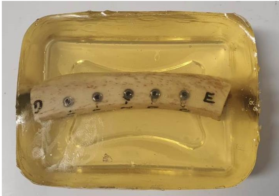
Figure1 - Image showing the bovine rib with the implants installed included in ballistic gelatin in order to simulate the soft tissues
