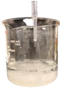
**Figura 18** – Intumescimento do PVA
