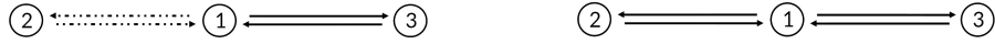
Figure 2 – (a) A 3-cell graph with distinct couplings and (b) a 3-cell graph with identical couplings.
