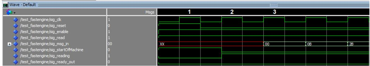
Figure 13 – Waveform showing how to write bytes with an external hardware.
