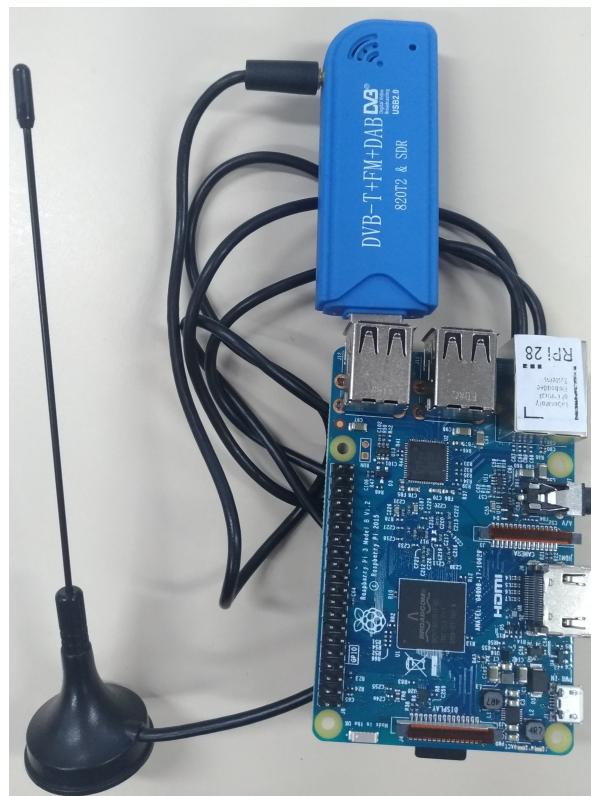
Figure 9 – CR platform built for this work. This is equipped with a basic antenna, an RTL SDR 820T2 as the radio front-end, and a Raspberry Pi 3.
