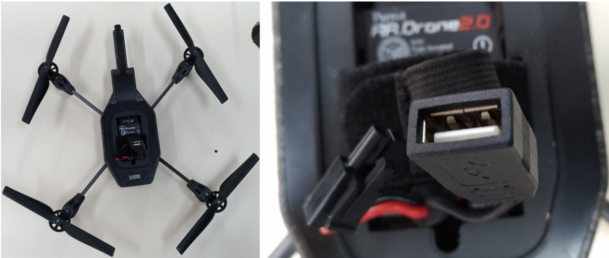
Figure 11 – The Parrot AR.Drone 2.0 without its hull, highlighting its USB port.
