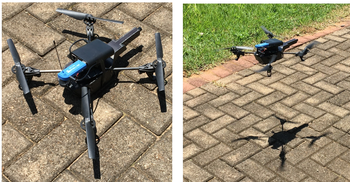
Figure 12 – The CR-based UAV testbed developed for this work. It consists of a Parrot AR.Drone 2.0 (Parrot, 2018a) UAV with a CR platform embedded to it.
