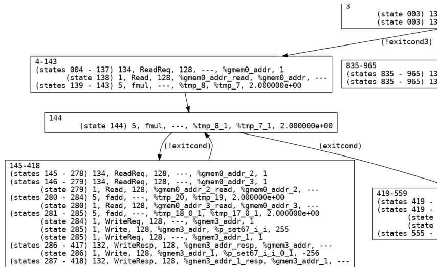
Figure 46 – Part of an FSM generated by vivado-fsmgen.
