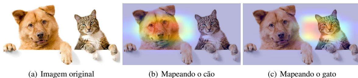
Figura 16 – Funcionamento do Gradient-weighted Class Activation Mapping (Grad-CAM).
