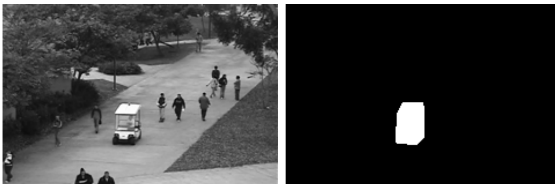
Figure 35 – An image from the Ped1 dataset containing an anomaly and its corresponding pixel-level ground-truth.
