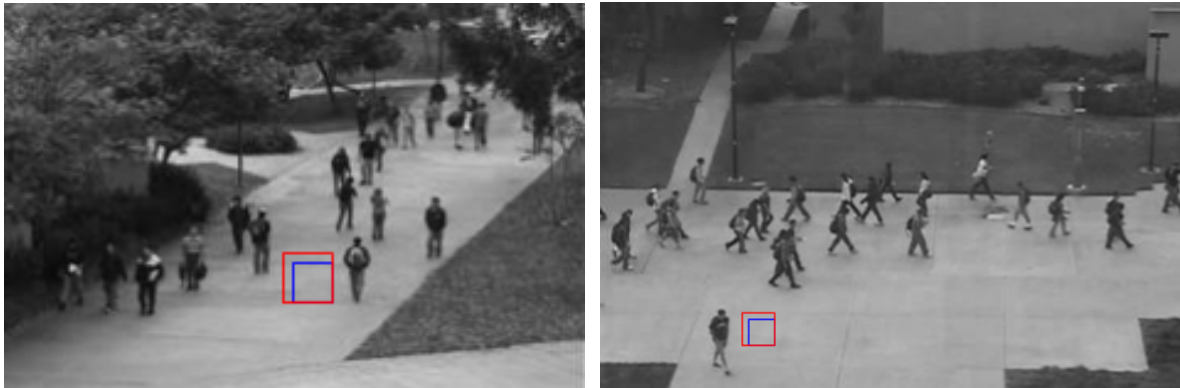
Figure 44 – Illustrating the base monitor size for the UCSD datasets: Ped1 (top), Ped2 (bottom). The blue and red bounding boxes represent monitor sizes equal to 16 and 20 pixels, respectively.
