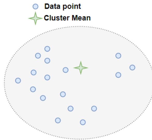
Figure 9 – An illustration about K-means clustering process. The centroid (green point) is the representative point of each cluster. The K-means algorithm assigns each incoming data point to one of the clusters by minimizing the sum in the cluster of squares.
