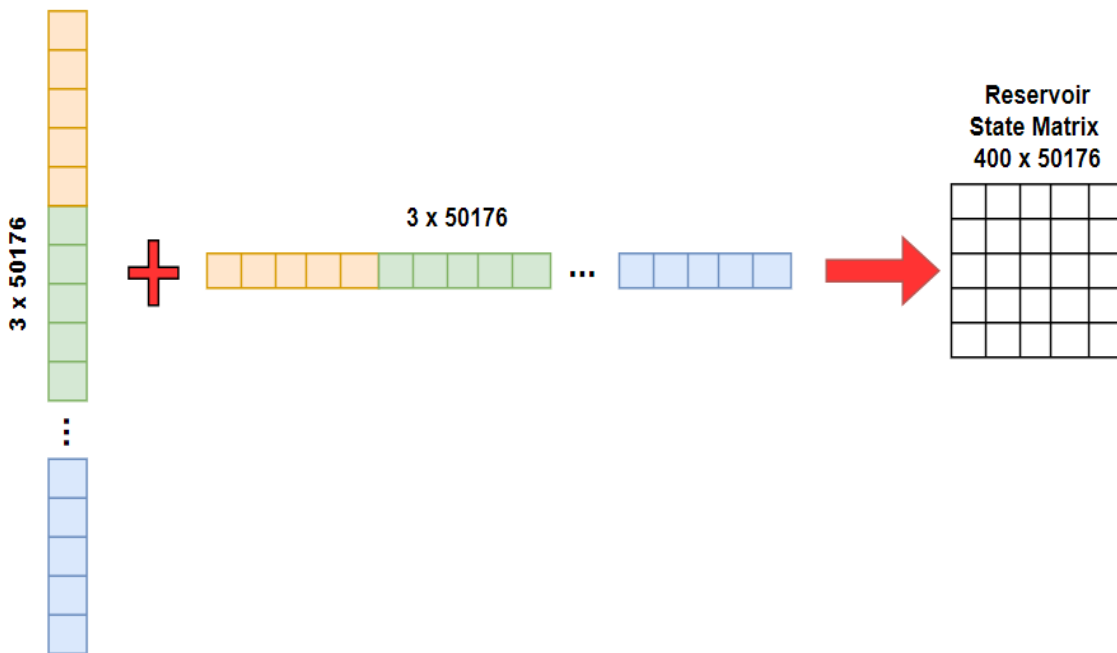
Figure 20 – First option of row-column concatenation process. The number of samples entering the network is doubled, since each vector is concatenated in both ways (by row and by column). Elaborated by the author.
