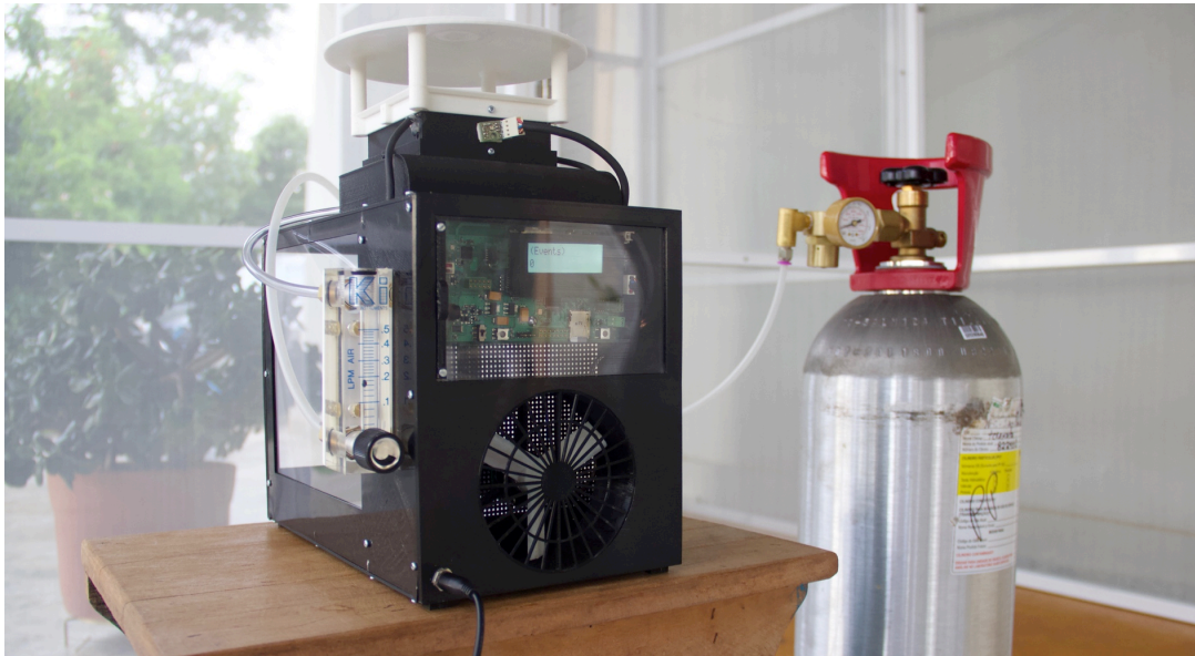
Figure 25 – The projected intelligent trap for flying insects.
