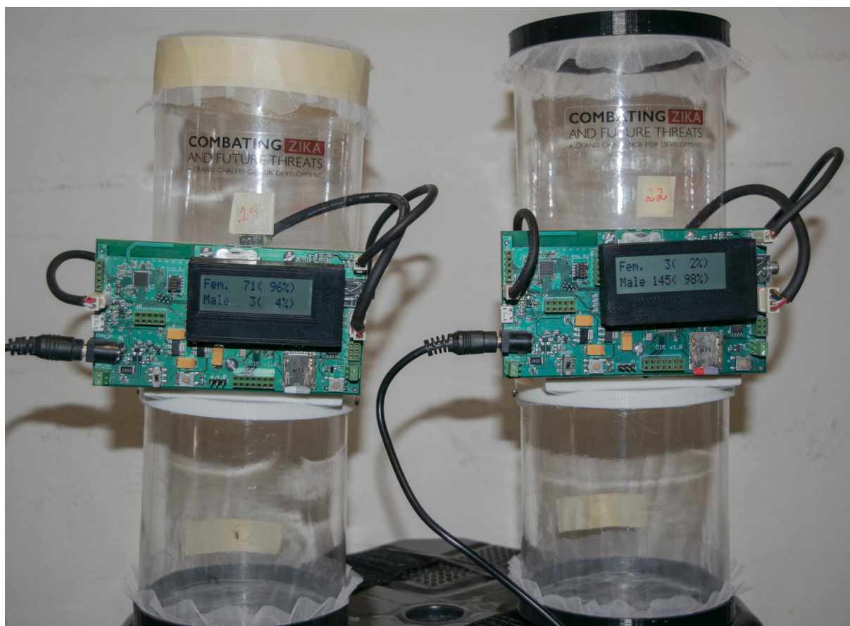
Figure 36 – Collectors used in the experiment. The left one contains five female Aedes aegypti mosquitoes and the right one contains five males.
