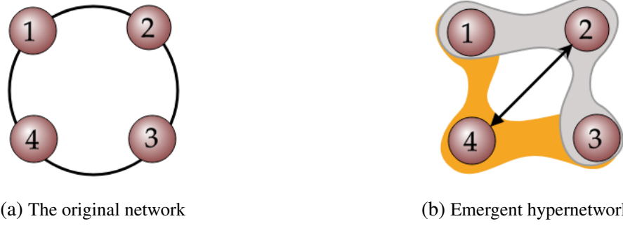
Figure 15 – (a) The emergent hypernetwork from the original ring network with a coupling function of the form h(z, w) = (z + z^2)\bar{w} . The frequencies \omega_k satisfy resonance conditions \omega_2 \approx \omega_1 + \omega_3 \approx \omega_4 . We also observe the emergence of diffusive coupling of oscillators 2 and 4.
