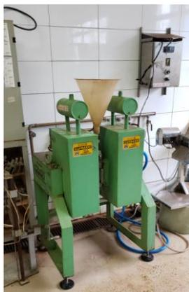
**Figura 7** – *Wet High Intensity Magnetic Separator* (WHIMS), modelo WHC-01 B
