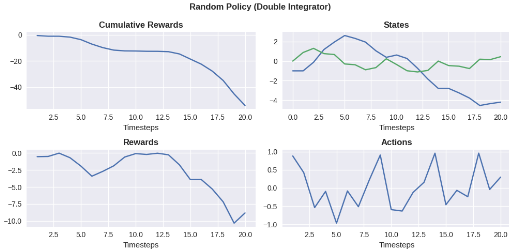
Figure 4.5: Double Integrator: a single run of a random plan. The system is quickly destabilized. In the top right chart, the velocity and the position of the system are given by the green and blue curves, respectively.
