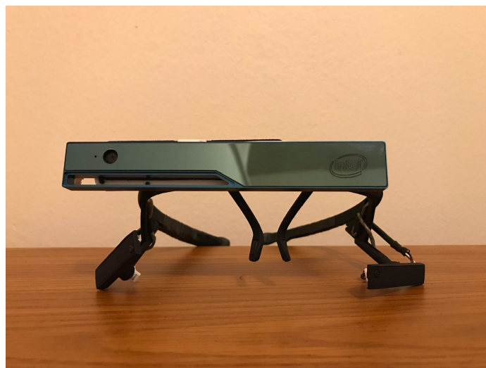
Figure 5.3: The Pupil binocular eye tracker coupled with an Intel Realsense R200 camera is used as a head-mounted setup.
