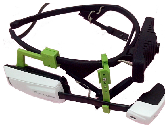
Figure 6.3: Prototype showing the Vuzix M100 Smart Glasses attached to a Pupil Labs head-mounted eye tracker using our custom mount.
