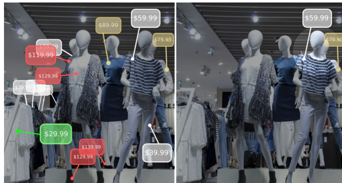
Figure 6.14: Augmented reality clutter (left), even when subjected to sorting and overlay occlusion mitigation, still may be perceived as AR pollution. Using gaze fixation (right), we correlate the relevancy of AR content to user attention, though triggering unwarranted AR content automatically just based on attention can be considered a form of the Midas touch problem.
