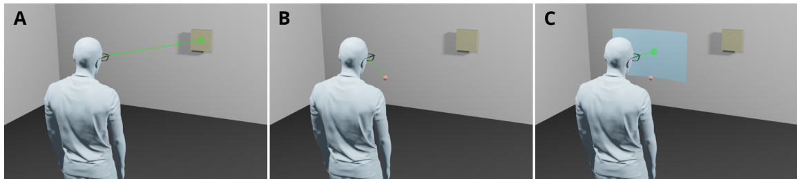
Figure 6.15: V-Switch Workflow. (A) Eye contact is established with a smart object, at a far distance. (B) A virtual point (the red dot) is rendered near the user, indicating that it is possible to interact with the object. To toggle the object's AR content, the user looks at the sphere. (C) V-Switch detects the vergence movement at the sphere and the interactive AR content is rendered.
