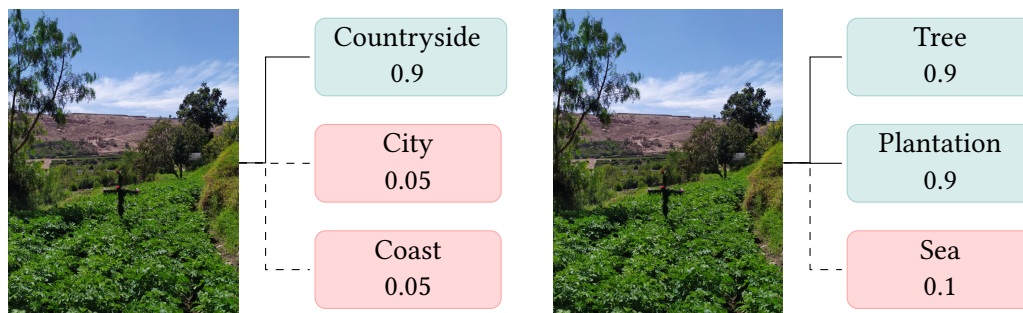
Figure 4.1: Example of multiclass (left) and multi-label classification (right)
