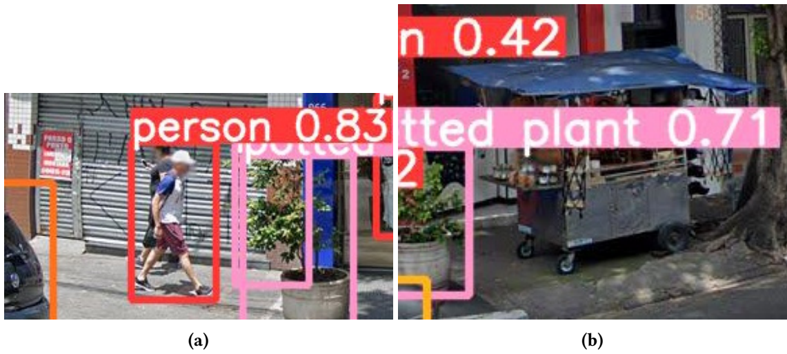
Figure 1.3: Details of the output of the YoloV5 for the image from the Rua Bresser. In (a) we see two persons detected as a single one, possibly due to occlusion. In (b) the YoloV5 failed to detect the food truck despite being in plain sight because there were no food trucks in its training dataset.
