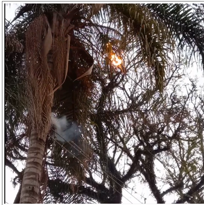
Figure 1.4: Electric arc formed by the contact of electrical wires with a tree.
