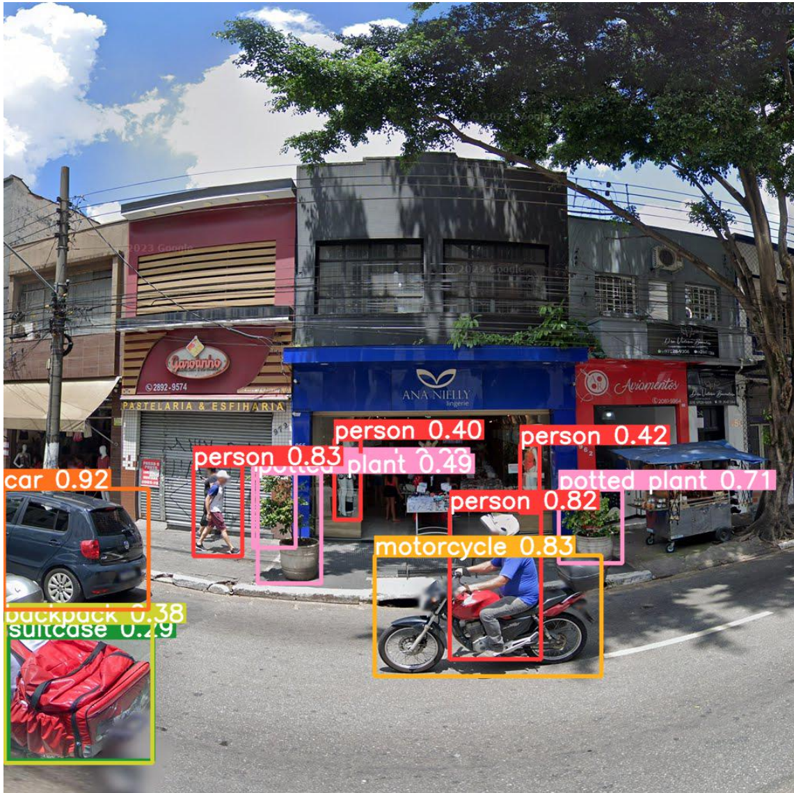
Figure 1.2: The output of a YoloV5 detection DLN. Notice that YoloV5 ignores trees, electric wires, building façades, poles, store signs, windows, and other elements despite being extremely common in urban scenes.
