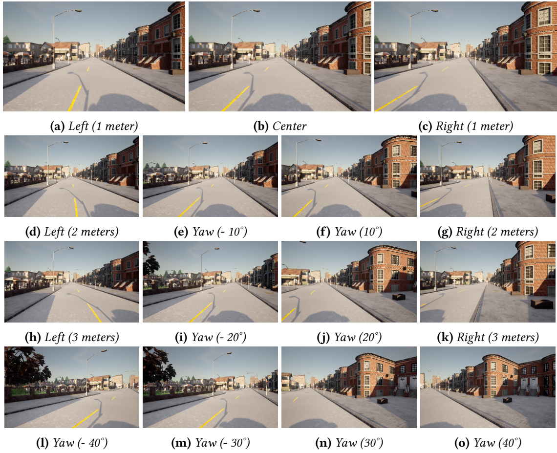
Figure 3.3: One shot at the same frame for all camera positions. The first model uses three cameras, (a), (b), and (c) of figure 3.3. The second model has seven attached cameras: the previous three cameras, plus (d), (e), (f), and (g). The third model increments four cameras, (h), (i), (j), and (k). Finally, the last model adds (l), (m), (n), and (o), totaling 15 cameras.
