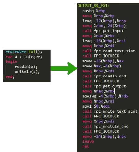
Figure 2.1: A program that reads an integer and prints it coded in Pascal and Assembly language
