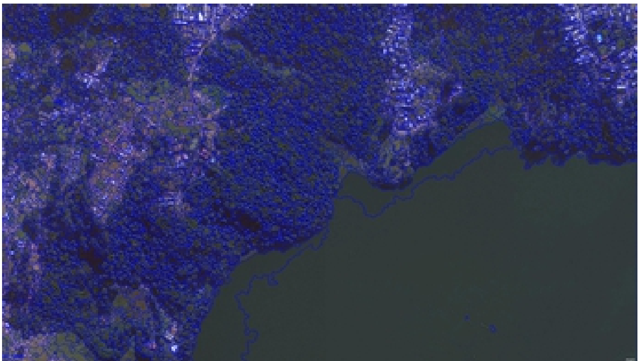
Figure 3.9: The output of applying spectral difference segmentation on Figure 3.8. Applying this segmentation step reduced The number of generated segments over the reservoirs significantly.
