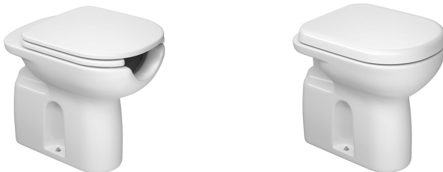
Figure 3.3: A breaking change in NBR 9050: the toilet bowl on the left has a frontal opening and was recommended in NBR 9050/2004 (ABNT, 2004). Even though this model is better for the hygiene of fully paralyzed individuals, it presents a risk of fall for more autonomous individuals. This was changed in the following edition (ABNT, 2015), which only recommends bowls without the opening, similar to the one in the right. Image source: (Deca, 2018).
