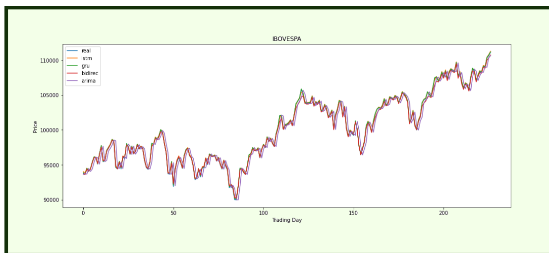
Figure 5.9: Sequence of real data and test data of the LSTM, BLSTM and GRU models, with lr=0.001 , batch size=10, number of epochs = 250 and 30 neurons of the four models for the Ibovespa index in the period from 21-12-2018 to 23-12-2019.
