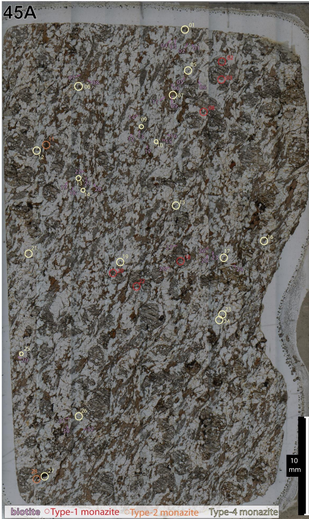
Figure 13. Location of biotite and monazite grains on thin section from the sample 45A under plane-polarised light.
