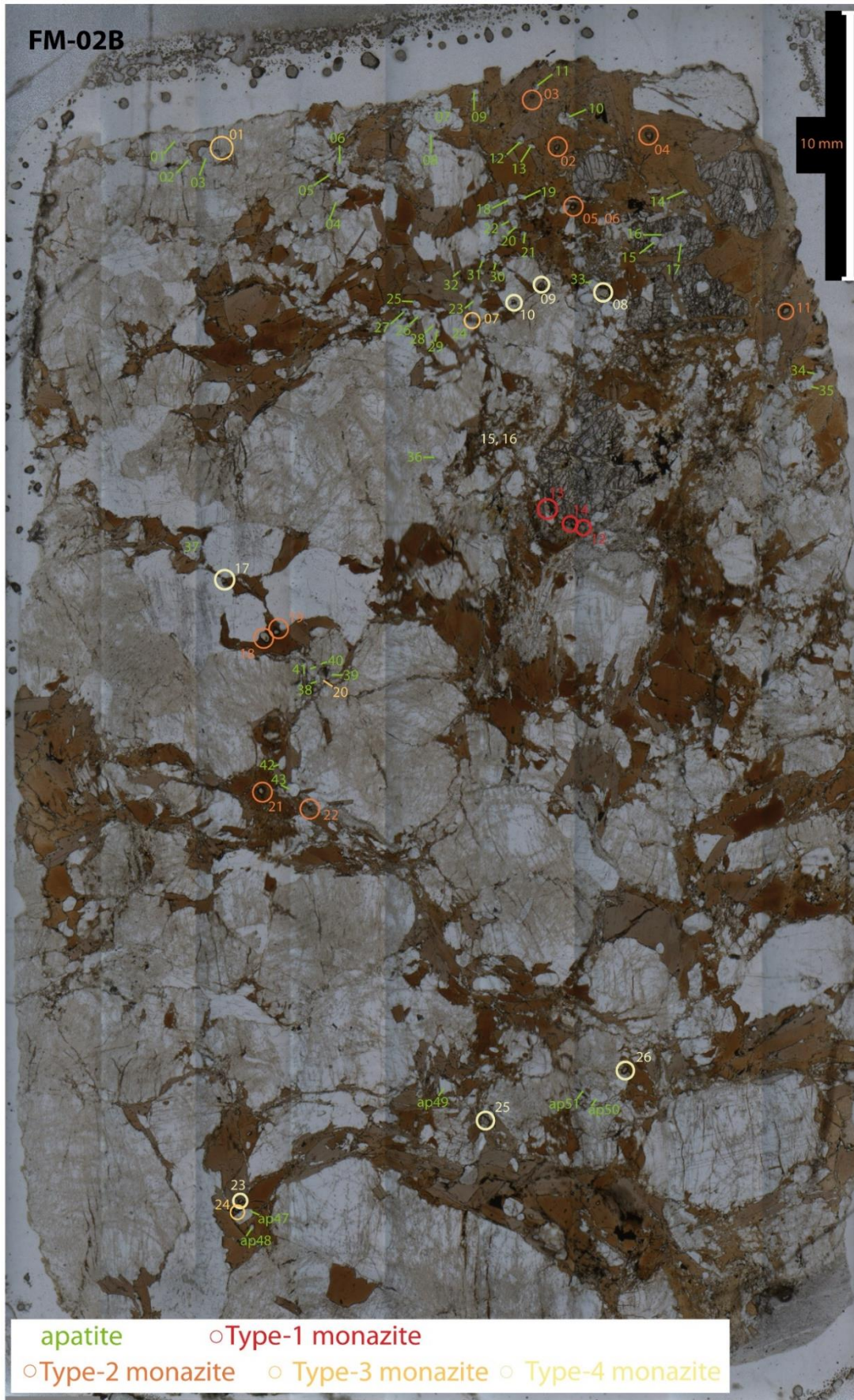
Figure 15. Location of apatite and monazite grains on thin section from the sample FM-02B under plane-polarised light.
