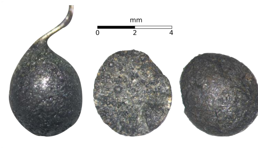
Figure 34 – Pictures of one of the microgabbro beads. Attached to the Pt wire (left); inner half (middle); outer half (right).
