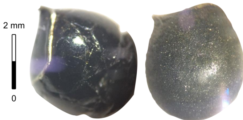
Figure 32 – Glass (left) and microgabbro (right) beads seen through a magnifying glass.
