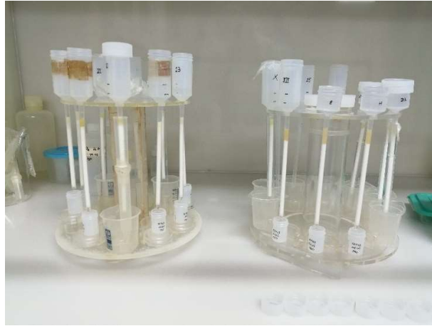
Figure 11. chemical separation of Nd element in column.
