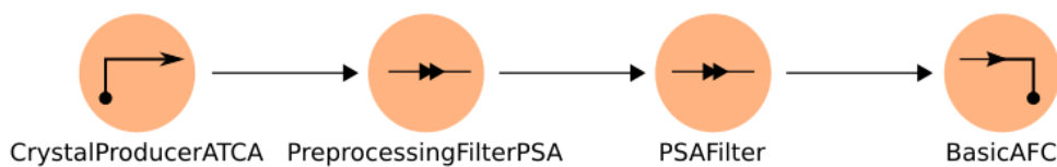
Figure A.2: Graphical representation of NARVAL topology file, with actor names. In this example, NARVAL reads the traces coming from the front-end electronics, then applies the pre-processing and PSA filters and after dumps the gamma-ray information into adf files. Adapted from [110].
